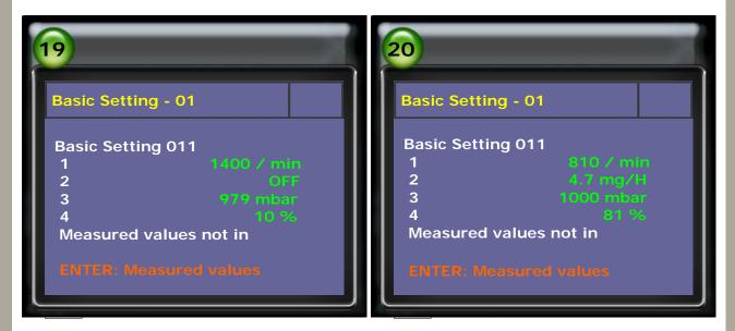
Enter the block number and access the basic setting, the 2 indicators on instrument cluster will light on (flickering) and the idling speed will also raise to approx. 1400 rpm.
