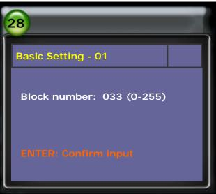
6. When entering 033, first press the brake pedal, then accelerator pedal. Both pedals must be pressed during basic setting. If not, the basic setting is aborted.
